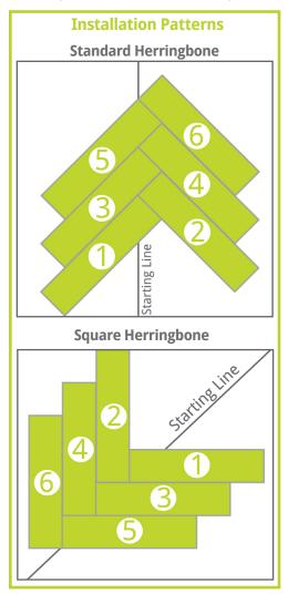
Determine the best wall to start the installation along – typically, this is the longest straight wall with a doorway. Measure the width of both ends of the room and, accounting for the necessary expansion gaps, calculate and mark the center of the installation area. Use a chalk-line to mark the center - this will serve as the starting line for the installation.
