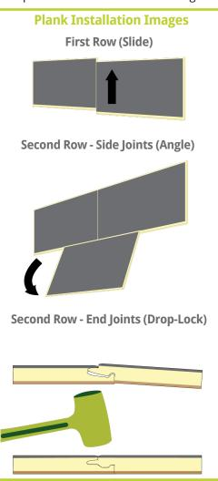
method. When you reach a doorway, make sure the cut edge will be covered by the door jamb and frame while maintaining the required expansion gap. Keeping the installation straight is critical - check the first row using a chalk line or similar and adjust or reinforce the entire row with wedge spacers as needed
