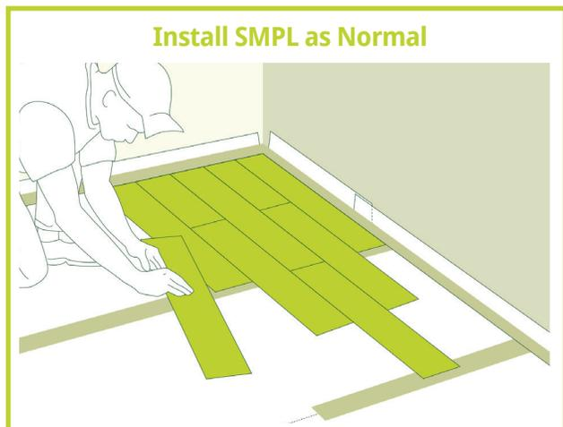
Once SMPL is completely installed, trim the overlap and any excess Endurance material around the perimeter to allow for the installation of wall base and/or any adjacent accessories or floor covering. Ensure that Endurance material still covers the entire installation area to ensure consistent sound reduction and moisture protection.
