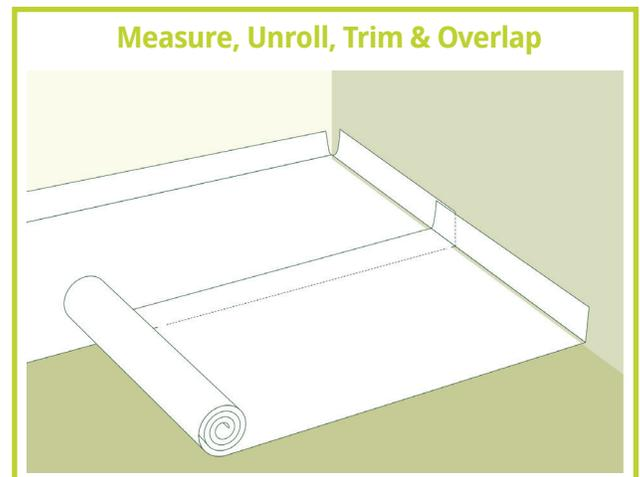
roll, ensuring the overlap is facing the same direction as the previous roll. Once seams are tight and in place, unfold the overlap to cover the previous roll and use 2" clear packaging tape to tape the overlap to the previous roll and the perimeter of the installation. Repair any tears or minor damage using a piece of 2" packaging tape as necessary. Proceed in this manner until the entire installation area is covered. Ensure there are no gaps whatsoever between each roll.
