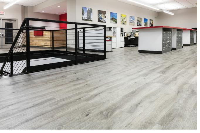
AVA® SMPL™ is our High Performance Core (HPC) luxury vinyl flooring with a commercial wear layer. It is a rigid and floating floor system that can be installed with minimal subfloor preparation. It is also waterproof and has an attached cork underlayment for improved acoustic performance.
